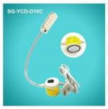
Model SG-YCD-D10C AC110V/220V/380V Input 0.8W Power LED 10pcsDIP 80lm Lumens CCT 6000-6500K Switch ON/OFF Installation Magnet Mounted Lifespan ≥50000 hrs
