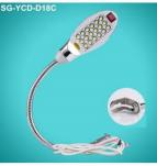
Model SG-YCD-D18C AC110V/220V/380V Input Power 1.3W LED 18pcsDIP 130lm Lumens CCT 6000-6500K Switch ON/OFF Installation Pitch Platet Mounted Lifespan ≥50000 hrs
